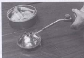
Exhibit 85. After a round sealed beam lamp is set to spinning on a smooth, level surface, a pencil-point propane torch flame can heat a circular strip on the reflector around the contact lugs.
